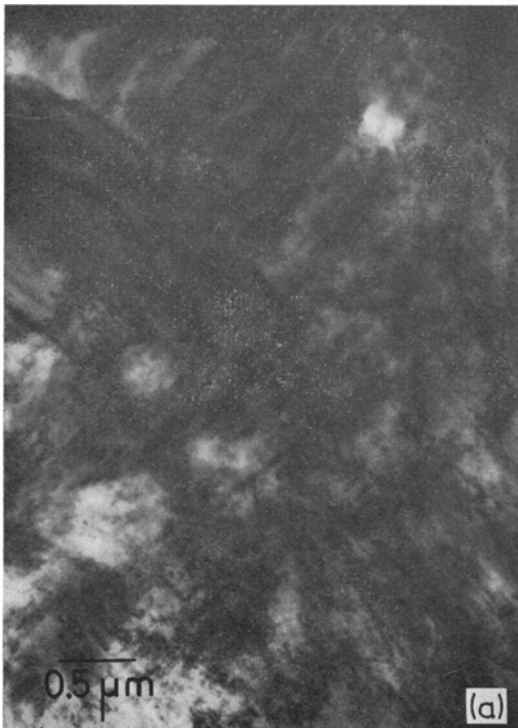
Figure 2 The solution-treated 50% cold-rolled condition aged at 175°C for (a) 2 h, (b) 24 h, (c) 100 h.
