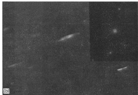
Figure 10 (a) \gamma' precipitates present in the solution-treated 50% cold-rolled material aged for 110 h at 425°C. (110) foil plane. (b) Dark-field micrograph of the (100)_{\gamma'} reflection.
